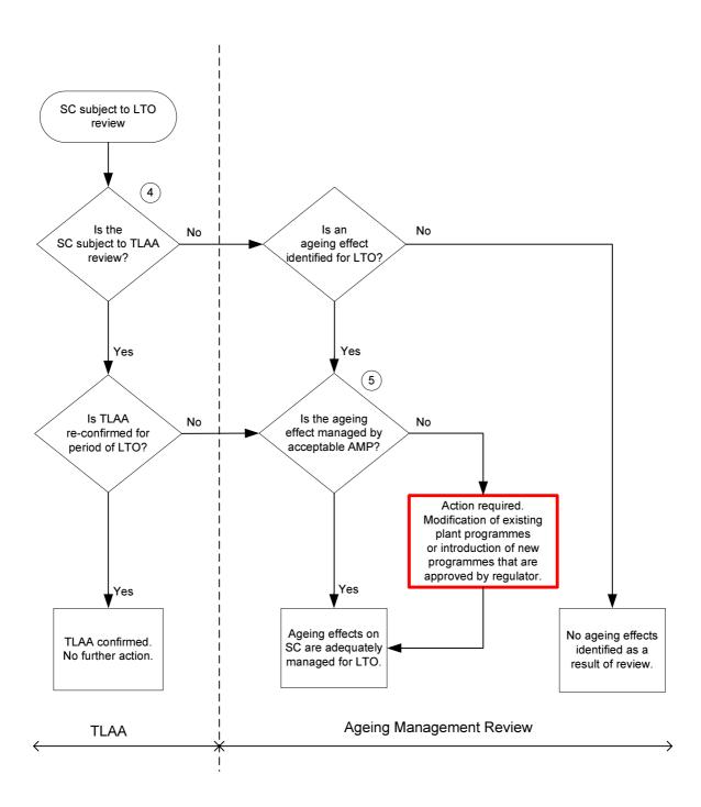
Fig.2. Screening Process for LTO
